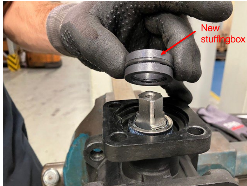
16) Place new Stuffingbox on top of graphite ring
